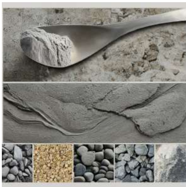
Fig. 2: A diagram showing the parts of concrete: cement, aggregate, water, and admixtures (pozzolans). Cement
