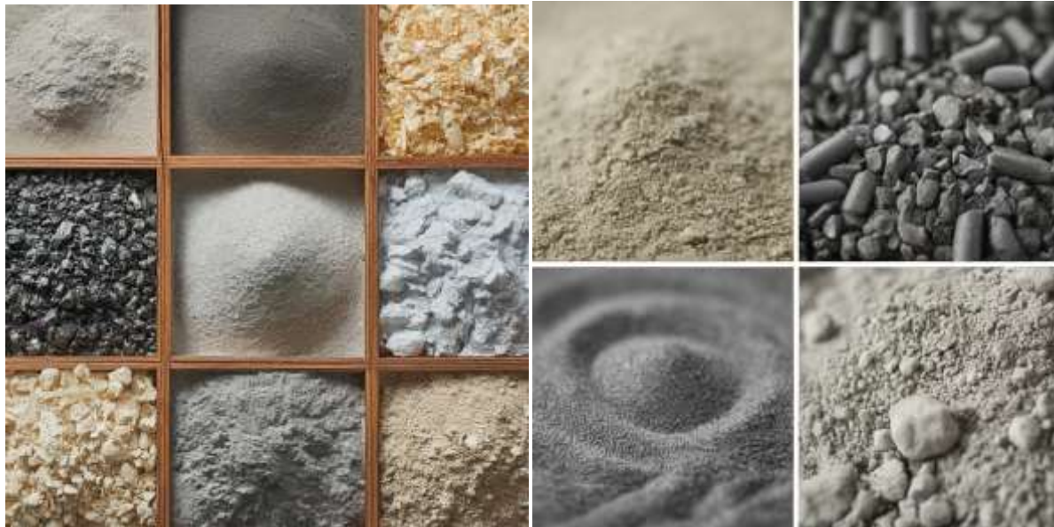
Fig. 1: Images display various mineral admixtures like fly ash, silica, ggbs, sawdust ash, and corn cob ash.
